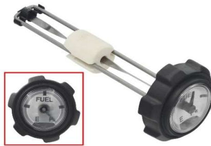
AT-07560 (LONG) L:198MM, CAP I.D: 52/58.2MM COLD RESISTANT -30 DEGREE C W/ INDICATOR, W/ NBR SEAL, W/ FUEL RESISTANT
